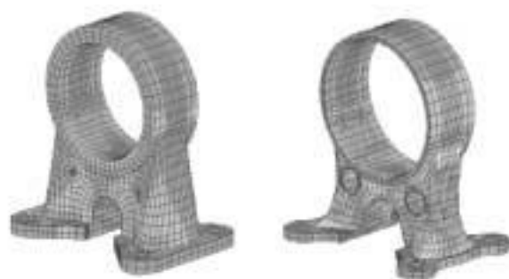
(a). Initial Shape (b). Optimum Shape
