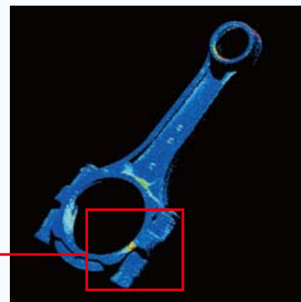
Extracted and highlighted flaw
