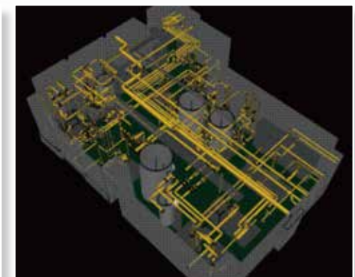
3D-CAD data created from the point cloud
