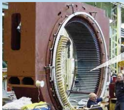
Optic fiber is attached to stator surface
